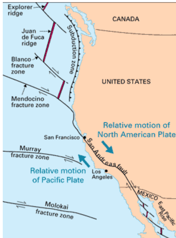
Fig. (2-20): The Blanco, Mendocino, Murray, and Molokai fracture zones are some of the many fracture zones (transform faults) that scar the ocean floor and offset ridges (see text). The San Andreas is one of the few transform faults exposed on land.
